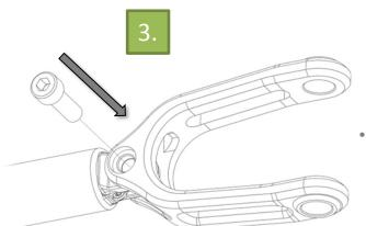
• Insert the M8 bolt and tighten with 14-16Nm
